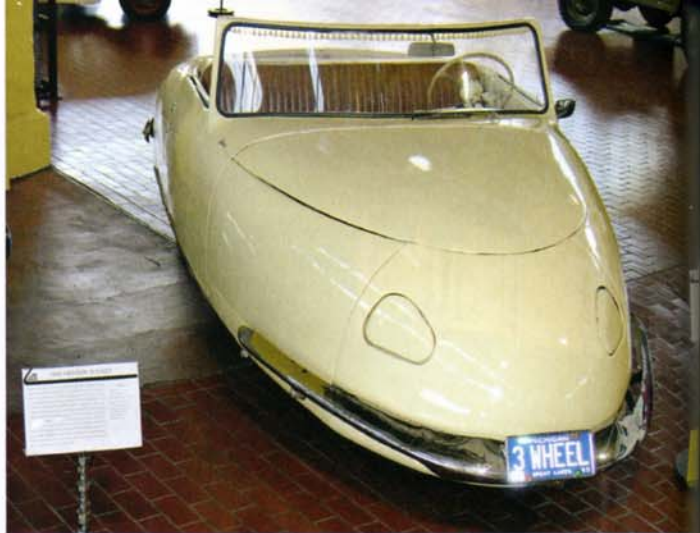
A removable hardtop, hidden headlamps and one front wheel are hallmarks of this Henry J-powered 1948 Davis Divan, one of 16 built
