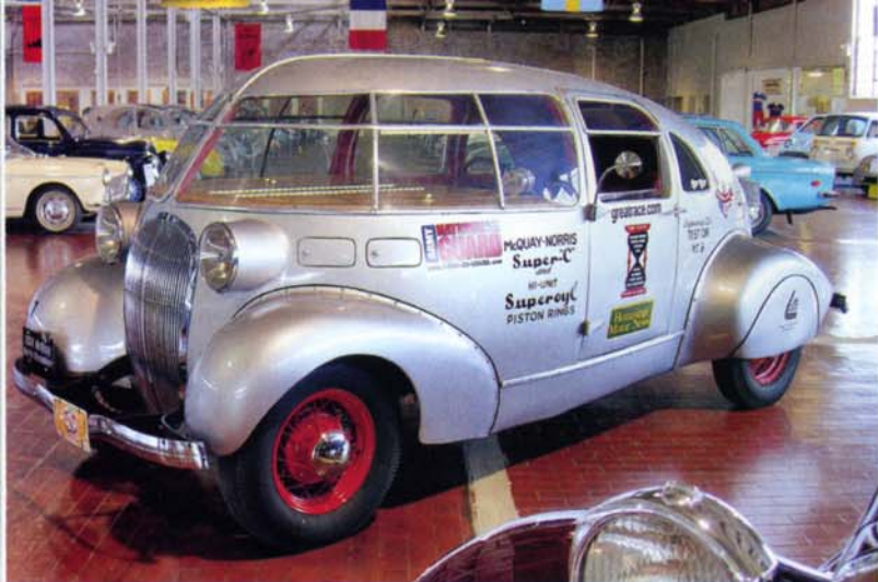
This 1934 McQuay-Norris Streamliner is one of six built by the eponymous St. Louis company; 85hp Ford flathead V-8 lets it hit 80 mph
