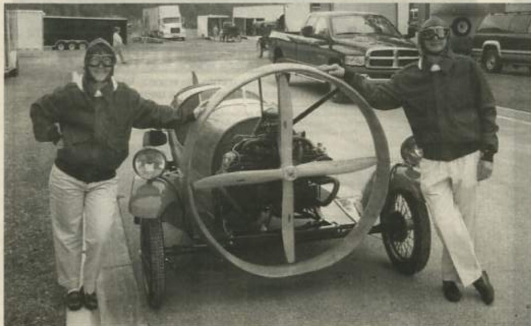
More of an airplane without wings than an automobile for the open road, the Helicron features a large four-blade propeller, an open cockpit, a stabilizer fin and rear-wheel steering.
